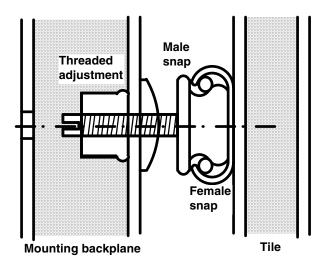
Figure 7. Adjustable tile mounting point.
