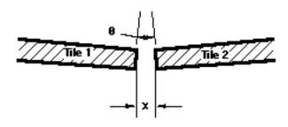
Figure 6. Tile-to-tile abutment and angular relationship.
