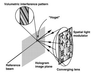
*Figure 2. General one-step, full-parallax holographic stereogram recording schematic.*
