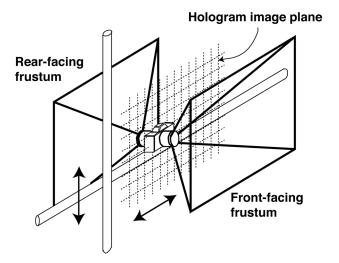
Figure 1. Hologram-centric double-frustum camera
