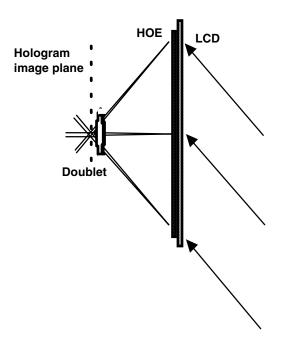
Figure 3. Optical printer mask beam elements.
